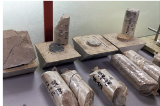
Drill core sample preparation for geotechnical experiment in the laboratory.
